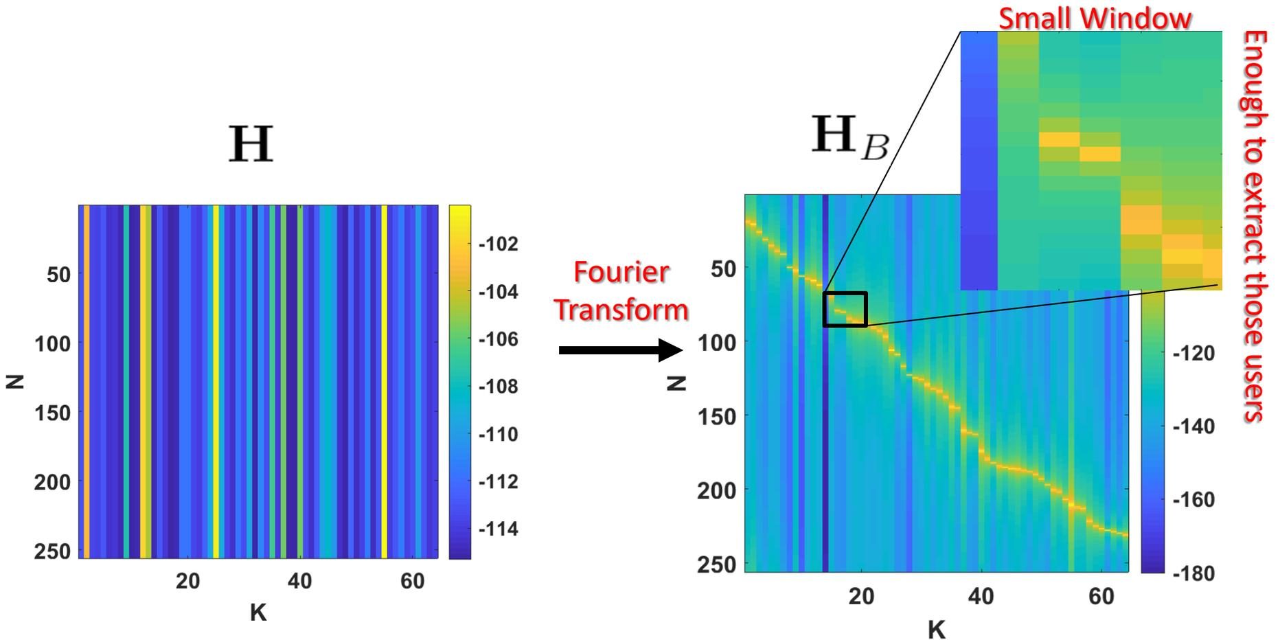
Most of the energy for a user can be captured in  $\sim 3$  FFT bins
