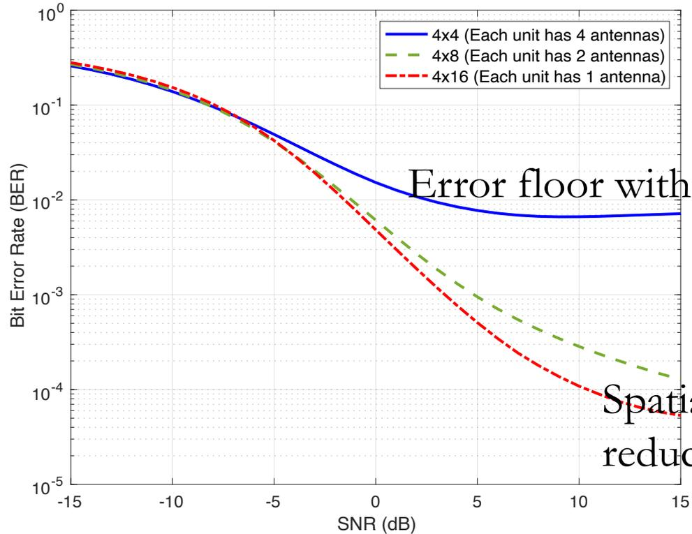
Error floor with array of subarrays
