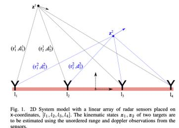
Fig. 1. 2D system model with a linear array of radar sensors placed on x-coordinates,  $\{l_1, l_2, l_3, l_4\}$ . The kinematic states  $z_1, z_2$  of two targets are to be estimated using the unordered range and doppler observations from the sensors.
