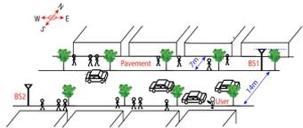
Fig. 1: Picocellular network deployed along an urban canyon
