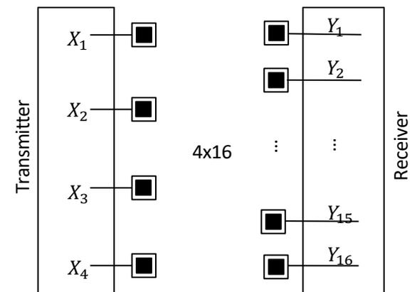
Each configuration has a total of 16 receive antennas.
