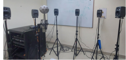
Fig. 5: Experimental setup for DOA estimation on real data in the lab environment.
