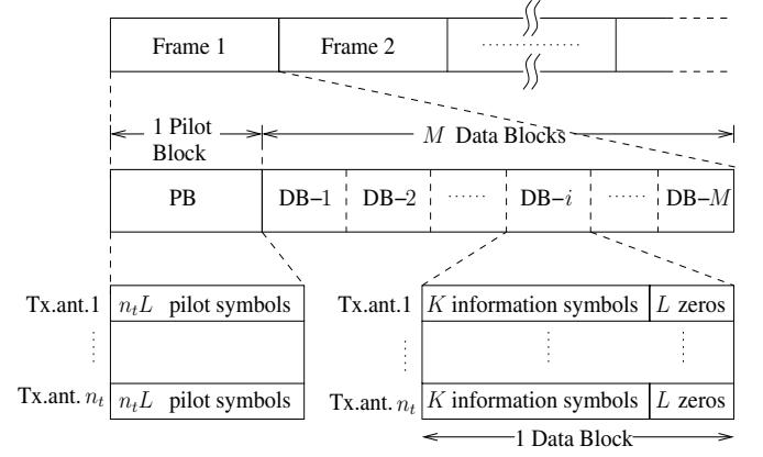
Fig. 1. Frame structure for MIMO-ZPSC system.
