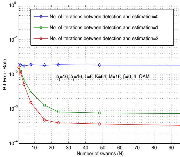
Fig. 5. Bit error rate of receiver as a function of number of swarms  $N$  for  $n_t = 16, n_r = 16, L = 6, \beta = 0, K = 64, M = 16$ , 4-QAM and SNR = 12 dB.
