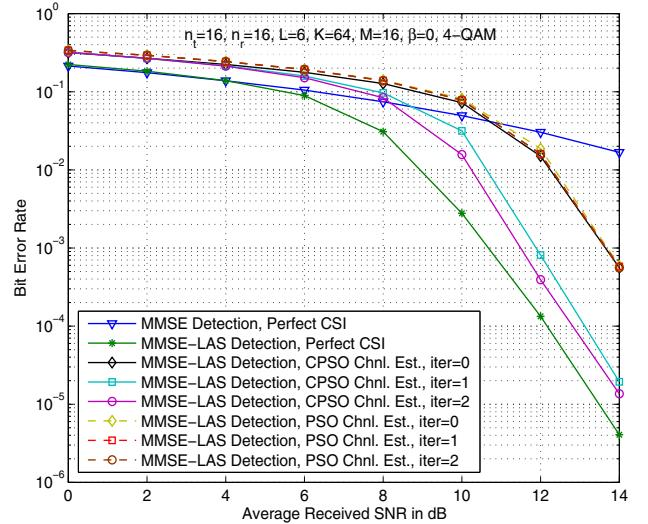
Fig. 3. BER performance of the receiver for different number of iterations between CPSO/PSO channel estimation and LAS detection for  $n_t = 16$ ,  $n_r = 16$ ,  $L = 6$ ,  $\beta = 0$ ,  $K = 64$ ,  $M = 16$ , 4-QAM.
