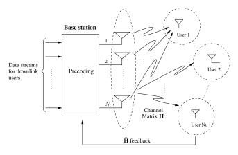
Fig. 1. Multiuser MIMO system on the downlink.
