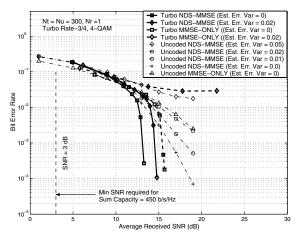
Fig. 4. Turbo coded BER performance of the proposed NDS-MMSE precoder without and with channel estimation errors.  $N_t = N_u = 300$ ,  $N_r = 1$ , rate-3/4 turbo code, 4-QAM. Sum rate =  $300 \times 2 \times 3/4 = 450$  bits/channel use.
