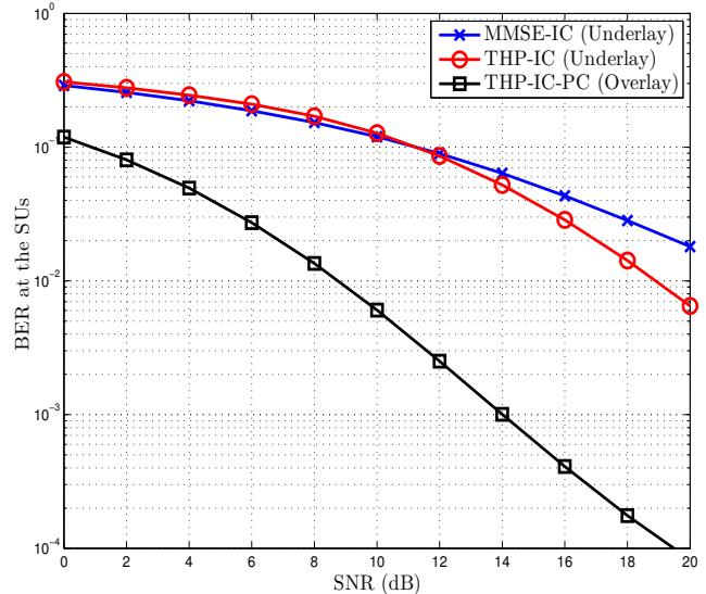
Fig. 4. Secondary User BER performance of the proposed precoding schemes at interference temperature  $\theta_i = -4.7$  dB,  $\forall i$ . PU SNR = 6 dB.  $R = N = 2$ ,  $M = 4$ ,  $K = 2$ . QPSK modulation.
