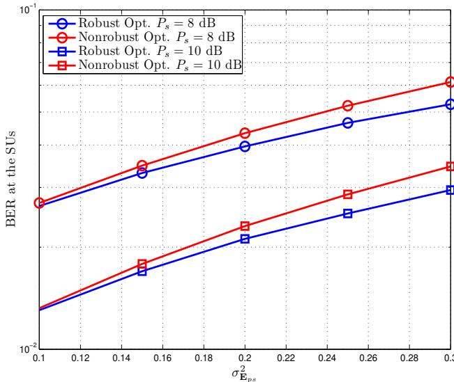
Fig. 6. Secondary User BER performance of robust and nonrobust precoding schemes with imperfect CSI for different values of  $\sigma_{E_{ps}}^2$ . Interference temperature  $\theta_i = -4.7$  dB,  $\forall i$ . PU SNR = 6 dB.  $\sigma_{E_{sp}}^2 = 0.01$ .  $R = N = 2$ ,  $M = 4$ ,  $K = 2$ . QPSK modulation.
