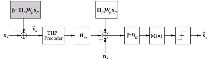
Fig. 3. THP at SBS with PBS data pre-cancellation (overlay model).
