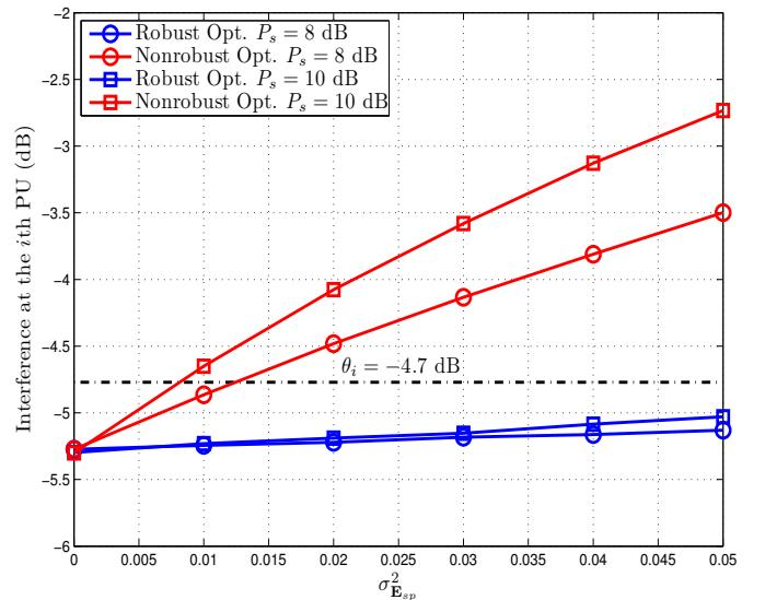
Fig. 7. Interference at the Primary User due to SBS transmission in robust and nonrobust precoding schemes for different values of  $\sigma_{E_{sp}}^2$ .  $\sigma_{E_{ps}}^2 = 0.1$ , interference temperature  $\theta_i = -4.7$  dB,  $\forall i$ . PU SNR = 6 dB.  $R = N = 2$ ,  $M = 4$ ,  $K = 2$ . QPSK modulation.
