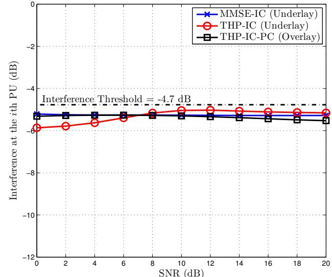
Fig. 5. Interference at the Primary User due to SBS transmission. Interference temperature  $\theta_i = -4.7$  dB,  $\forall i$ . PU SNR = 6 dB.  $R = N = 2$ ,  $M = 4$ ,  $K = 2$ . QPSK modulation.
