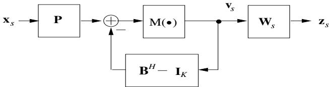
Fig. 2. Proposed THP precoder at the SBS with interference constraints.
