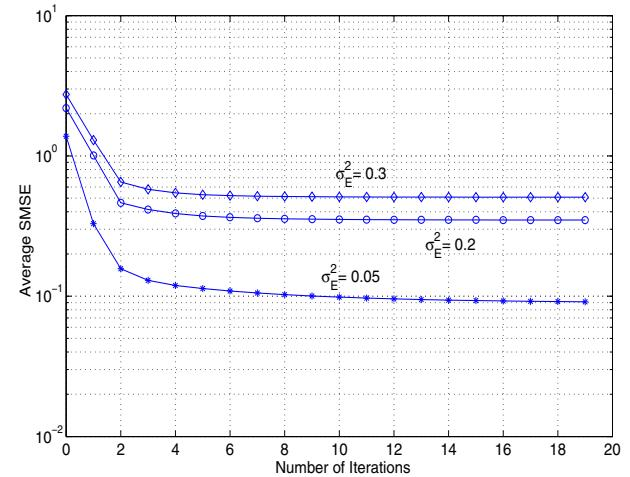
Fig. 3. Convergence behavior of the proposed robust transceiver design for different CSI error variances,  $\sigma_E^2 = 0.05, 0.2, 0.3$ .
