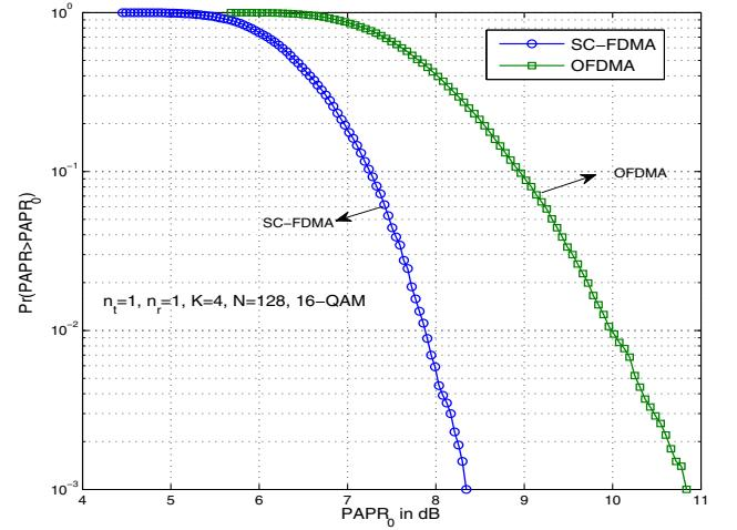
Fig. 3. PAPR performance of multiuser SISO SC-FDMA and OFDMA for  $n_t = 1, n_r = 1, K = 4, N = 128$ , 16-QAM.
