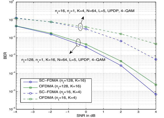
Fig. 8. BER performance of large-scale multiuser MISO downlink SC-FDMA and OFDMA for *i*)  $n_t = 16, n_r = 1, K = 4, L = 5$ , 4-QAM, and *ii*)  $n_t = 128, n_r = 1, K = 16, L = 5$ , 4-QAM.
