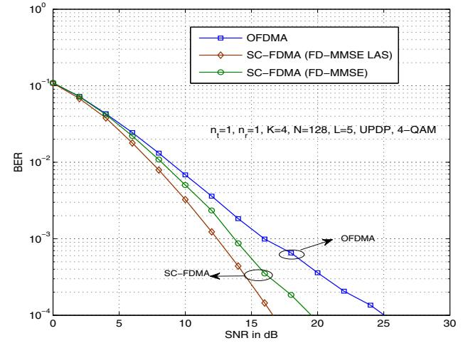
Fig. 4. BER performance of multiuser SISO downlink SC-FDMA and OFDMA for  $n_t = 1, n_r = 1, K = 4, N = 128, L = 5$ , 4-QAM.
