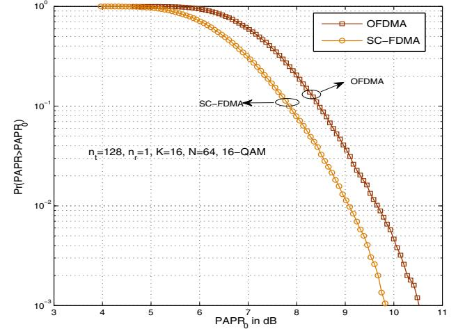
Fig. 7. PAPR performance of large-scale multiuser MISO SC-FDMA and OFDMA for  $n_t = 128, n_r = 1, N = 64, K = 16$ , 16-QAM.
