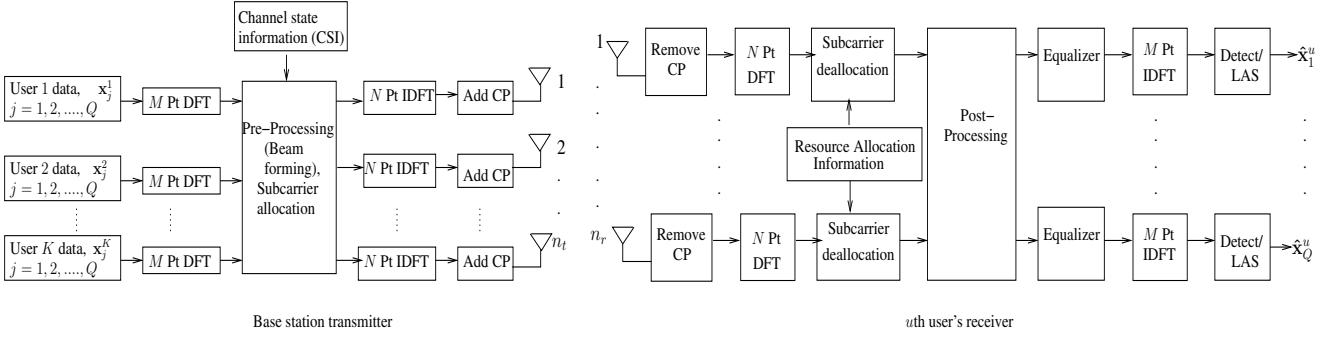
Fig. 2. Transmitter and receiver block diagrams of MIMO SC-FDMA on the downlink.
