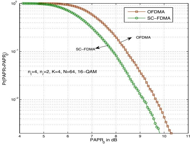
Fig. 5. PAPR performance of multiuser MIMO SC-FDMA and OFDMA for  $n_t = 4, n_r = 2, K = 4, N = 64$ , 16-QAM.
