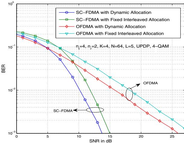
Fig. 6. BER performance of multiuser MIMO downlink SC-FDMA and OFDMA for  $n_t = 4, n_r = 2, K = 4, N = 64, L = 5$ , 4-QAM.
