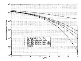
Fig. 6. BER performance of 16-QAM with different STBCs -i) 2 Tx antennas using rate-1 STBC (Alamouti code), ii) 3 Tx antennas using rate-1/2 STBC, iii) 5 Tx antennas using rate-7/11 STBC. Number of receive antennas,  $L_2 = 2$ .
